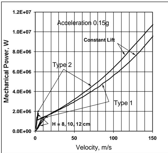
Fig. 8 Mechanical Power for a 25 t Vehicle Using either Type 1 or Type 2 Modules
