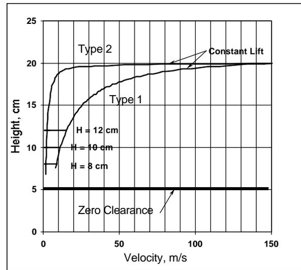
Fig. 5 Height vs. Speed Performance for Module Types 1&2
