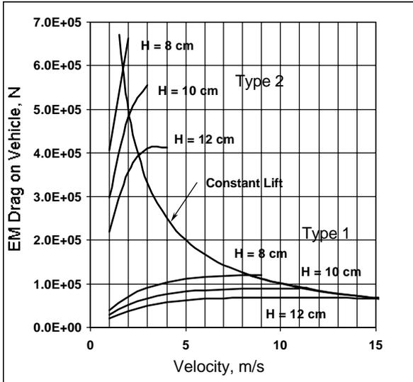
Fig. 7 EM Drag for a 25 t Vehicle Using either Type 1 or Type 2 Modules at Speeds below 15 m/s
