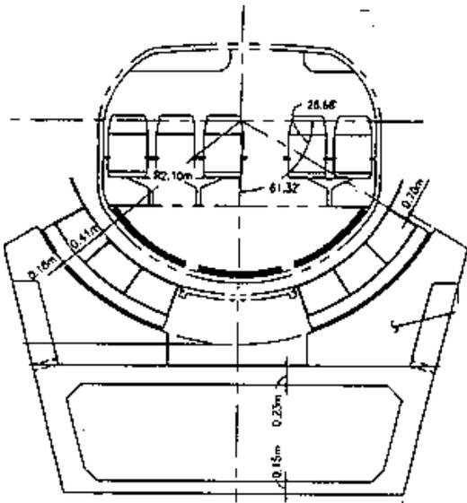
Fig. 2: Cross-section of vehicle, reinforced aluminum guideway and auxiliary long-span pre-tensioned concrete beam support
