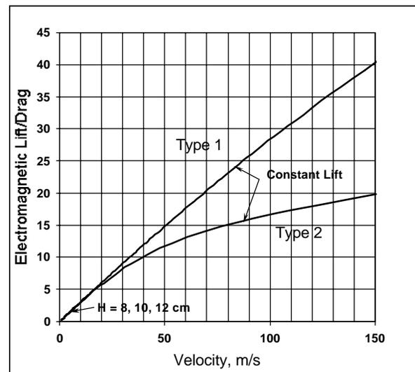
Fig. 6 Ratio of EM Lift/Drage for Module Types 1&2
