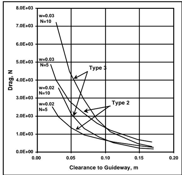
Fig. 10 Drag per Module vs. Clearance above Guideway
