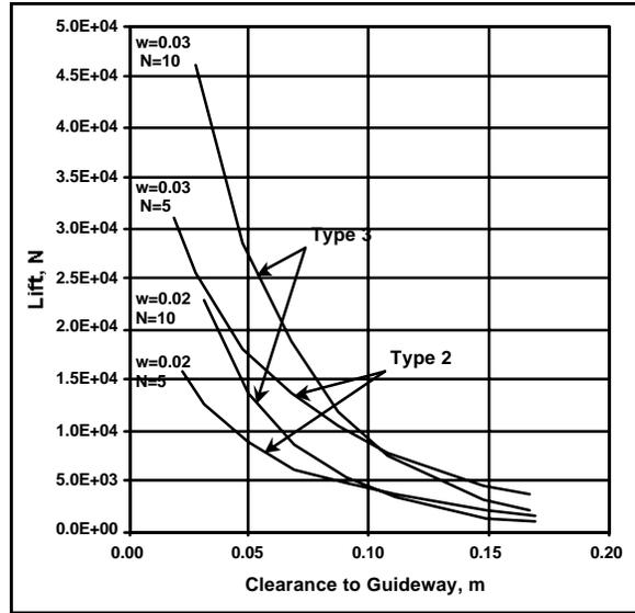
Fig. 9 Lift per Module vs. Clearance above Guideway
