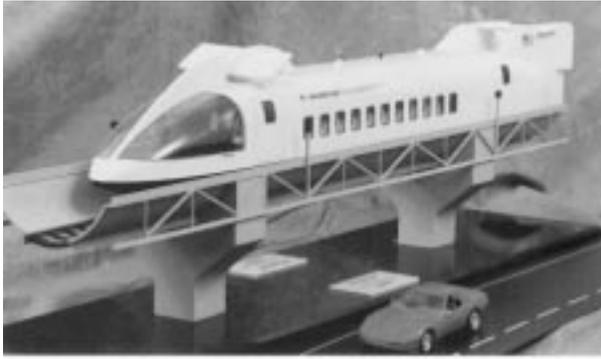
Fig. 1: Model of Magplane 25 tonne vehicle on aluminum sheet guideway
