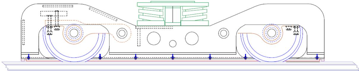
Fig. 6. The side view of light bogie with mounting Halbach-array permanent magnets
