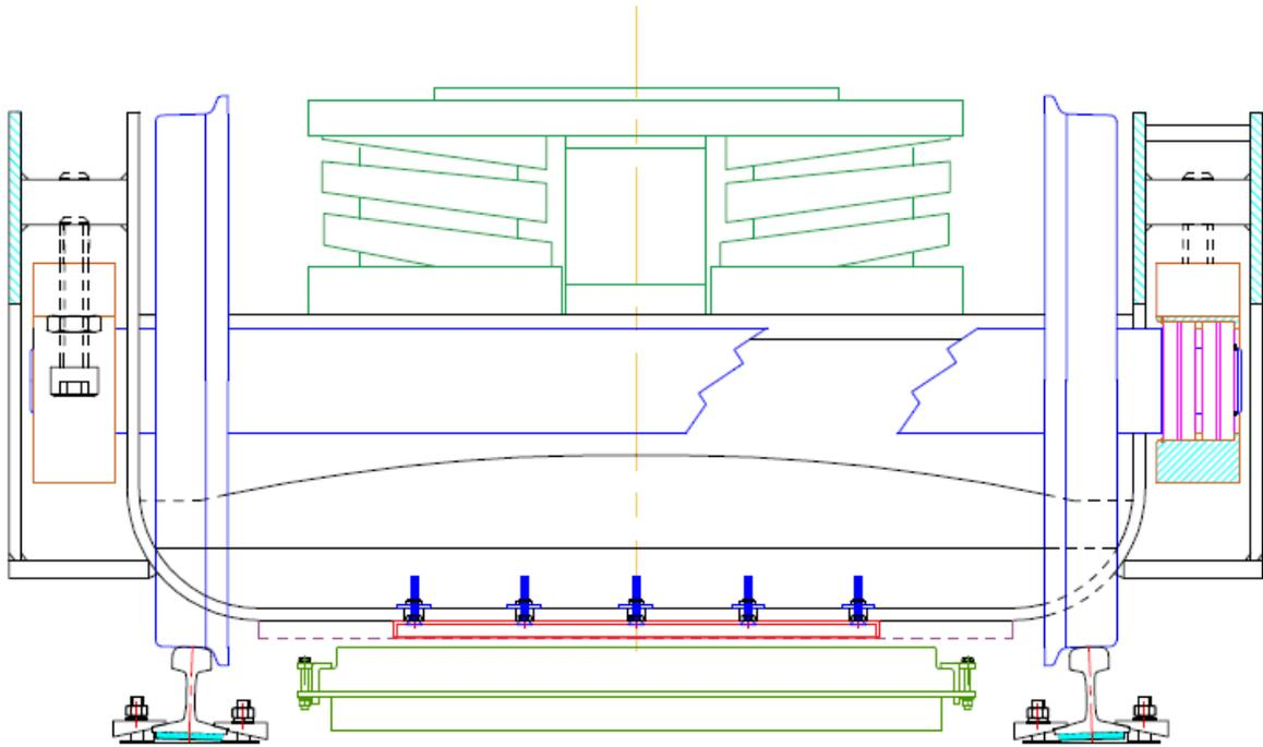
Fig. 5. The front view of light bogie with mounting Halbach-array permanent magnets
