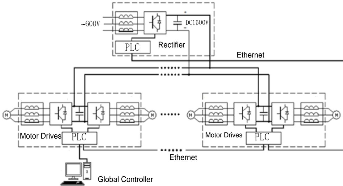
Fig. 7. Scheme of common DC Bus power for motor drives
