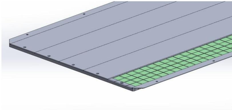
Fig. 4. Typical assembly of Halbach-array permanent magnets
