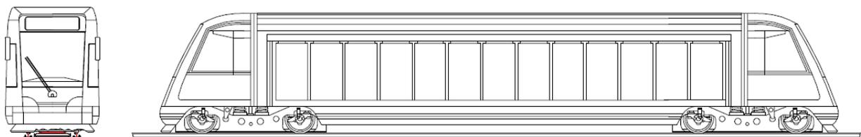
Fig. 1. A single 20m-long MagTrain vehicle with 2 magnet arrays attached on bogies
