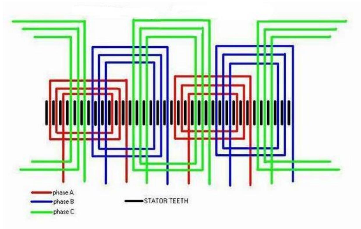
Fig 2. Three-phase, four-pitch windings scheme of MagTrain LSM
